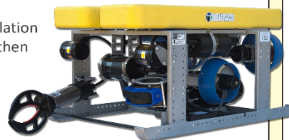
The Outland Technology ROV-2500, which is being used to record video footage for relative abundance indices.
